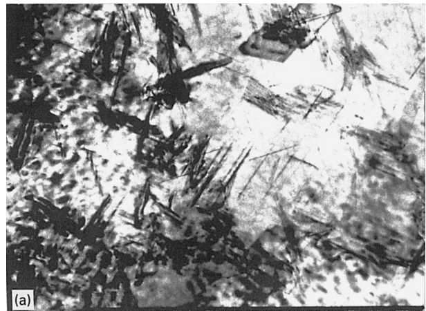
Figure 5(a) BF micrograph of S' rods grown along three \langle 100 \rangle matrix directions. Magnification \times 38000 ; (b) associated SAD pattern indicating [001] zone axis.
